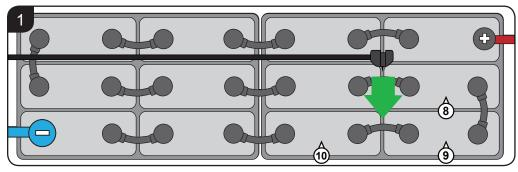
Black wire - attach to an intercell connector at least 8 cells from the positive take off.
