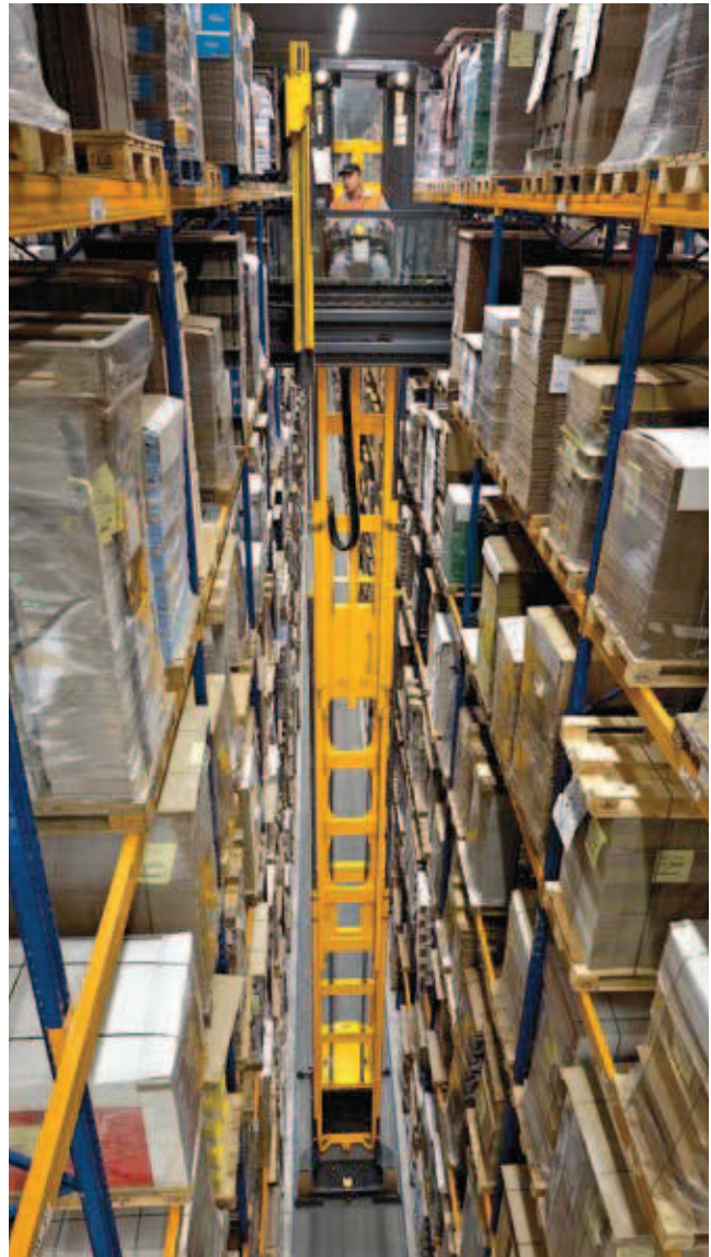
EKX 515, lifting height 16.5 m
